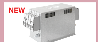
FMBD NEO: Terminals for 3 phases, neutral conductor and ground, intended for use in 4 wire systems. 8-200A, 300/520 VAC, screw clamp terminals
