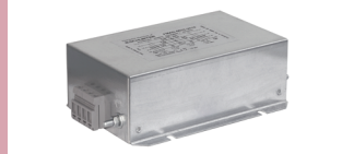
FMAD: High current filter w/neutral conductor, approved for high temperature applications, 6-550A, 275-480 VAC, screw clamp terminals
