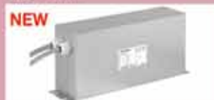
FMAC SINE DCL: Sine wave output filter, features DC link circuit, allows motor cables up to 1000m under full load. 4-16A, 500/288 VAC
