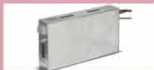
FMBC Book Style: Very compact slim filter for frequency converters and inverters 10-115A, 480 VAC, screw clamp / flexible wire terminals
