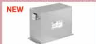
FMAC SINE: Sine wave output filter, allows motor cables up to 200m under full load. 4-16A, 500/288 VAC, screw clamp terminals
