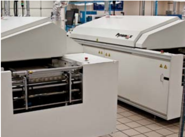
Zoned ovens ensure control over solder reflow
