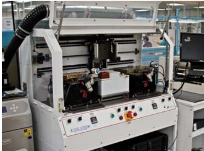
Automated solder dip equipment
