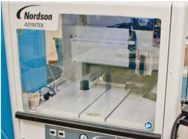
Automated potting controls process and quality
