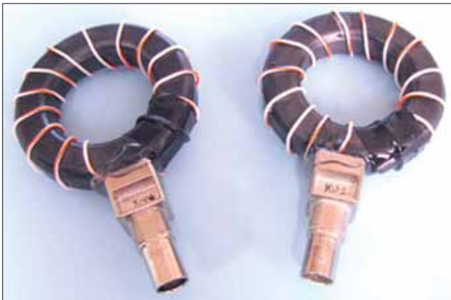
Figure 4. Examples of DIY current probes based on a large toroid core. These photos were taken prior to installing the E-field shield which consists of a layer of copper tape over the windings, leaving a small gap around the inside of the toroid. 14 turns of Teflon-insulated wire wound around a Würth Elektronik #74270097 ferrite core (4W620 material) was used, which is useful from 10 to 1000 MHz.
