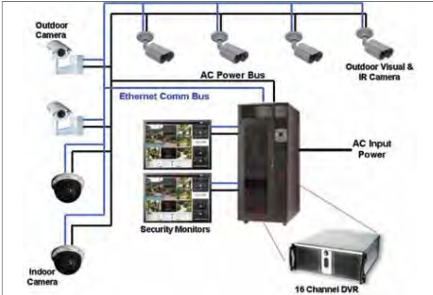
Figure 3. Overview of a security system.
