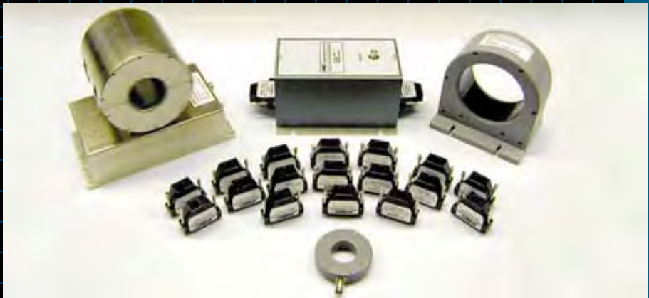
CISPR-22 Telecom Conducted Emission Test Accessories
