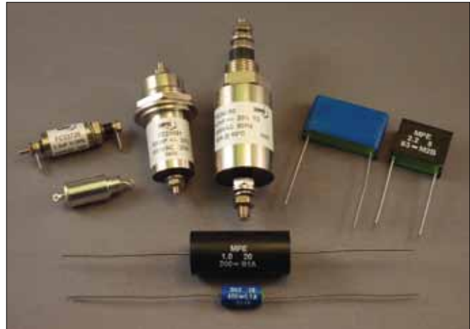
Figure 2. Typical feedthrough capacitors compared with two-terminal capacitors.
