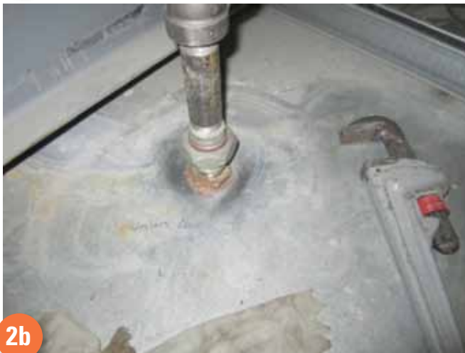
Figure 2. Condition of sprinkler condition at top of chamber. (a) Corrosion at one of the waveguides on top of the chamber. (b) The same waveguide after cleaning. Brass wool can be seen between the waveguide nut and the chamber surface.
