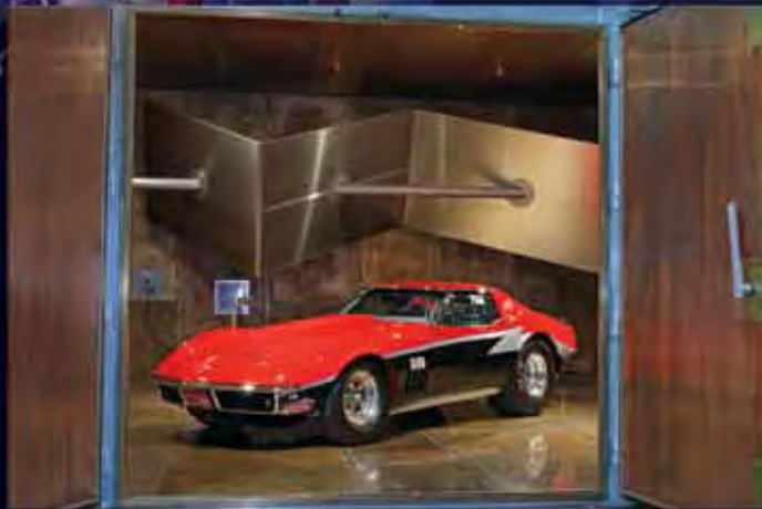
Full size automobile inside 25' x 30' x 14' Mode Tuned Chamber
