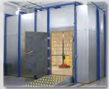
3 Meter EMC Chamber
