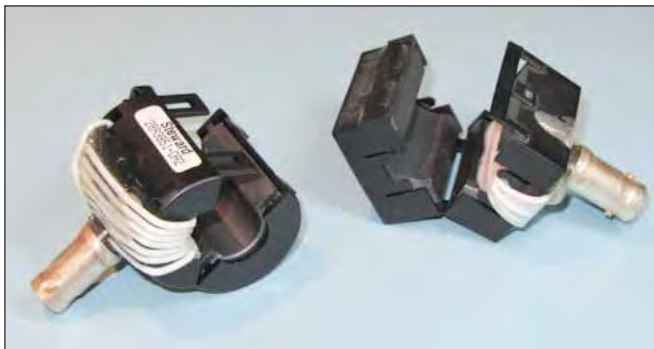
Figure 5. Examples of DIY current probes based on clamp-on ferrite chokes. I used a couple sample Steward (now a unit of Laird Technologies) chokes – a round one (model 28A3851-0A2) and a square one (model 28A2024-0A2). They each had 7 turns of Teflon-insulated wire wound around one-half and glued down on the inside to hold the windings. I later epoxied a PC board-style BNC connector to the outside, making sure there was enough epoxy to hold the outer turns together. Type 28 material was used, which is useful from 10 to 1000 MHz.
