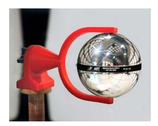
FIGURE 1 – USDS and Tripod Yoke Mounting Assembly
