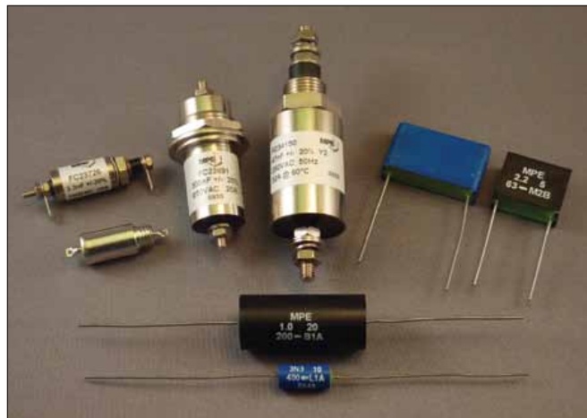
Figure 2. Typical feedthrough capacitors compared with two-terminal capacitors.
