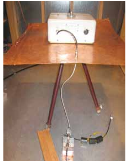
Figure 6b. MIL-STD-461F configuration using isolation XFMR visible near floor ground point. Assembly to the right is the rf sleeve network that gave the plot of Figure 5a.
