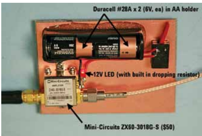
Figure 5. I made my own broadband preamp using a Mini-Circuits model ZX60-3018G-S. It is powered it with two 6V Duracell #28A batteries, which happen to fit in a standard “AA” battery holder. The amplifier covers 20 to 3000 MHz at 20 dB gain and is used to boost the probe signals.
