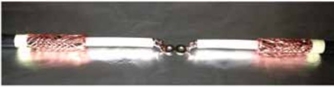
Figure 5. Grounded DUT hook-up test leads.
