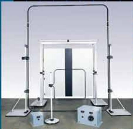
IEC 1000-4-8 Test Equipment
