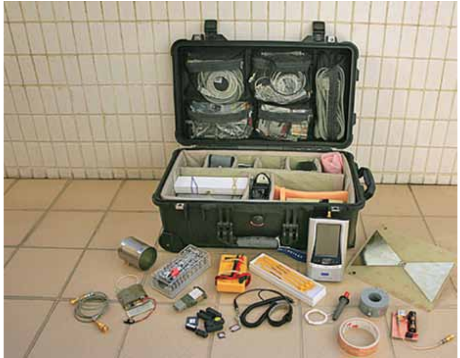
Figure 12. Contents of the special EMC troubleshooting kit I've assembled. I can probe for various RE problems, as well as test for ESD and radiated immunity. Performing these tests early in the design cycle, results in a greater chance of passing the required EMC product qualification tests.
