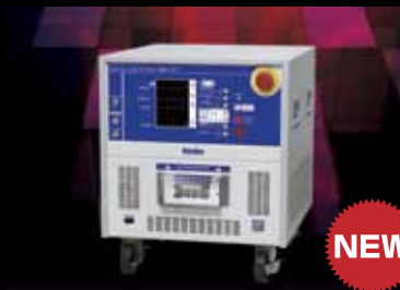
Lightning Surge Simulator-Compact type LSS-6230 Conforms to IEC-61000-4-5 (1.2/50; 8/20µs) ANSI/IEEE C62.45 Ring Wave (0.5µs-100kHz) Max. voltage 6.6kV
