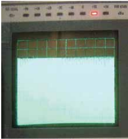
Figure 4a. Rf potential on radiating wire loaded by 50 Ohms. Span is 2-32 MHz, reference is 10 dBm, 10 dB per division (-10 dBm = 97 dBuV).
