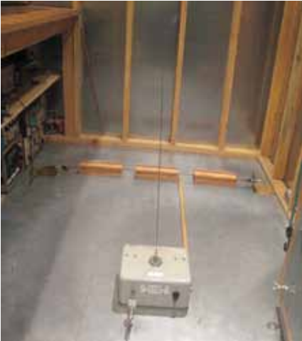
Figure 7a. "Reality" check configuration. Separation of radiating line from back wall the same as when on table-top ground plane.
