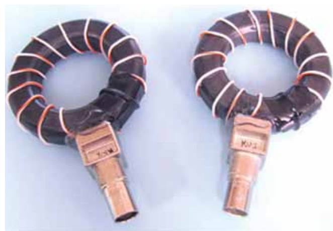
Figure 7. Examples of DIY current probes. These photos were taken prior to installing the E-field shield by wrapping a layer of copper tape over the windings, leaving a small gap around the inside of the probe. 14 turns of Teflon-insulated wire wound around a Würth Elektronik #74270097 ferrite core (4W620 material) was used, which is useful from 10 to 1000 MHz.
