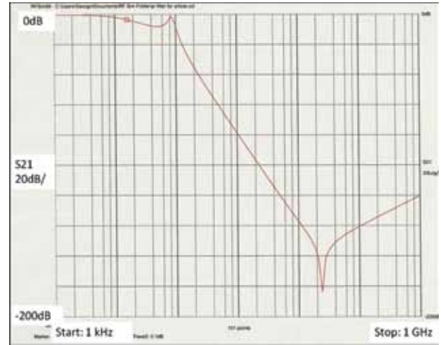
Figure 11. .22μF/40μH/.22μF Filter Insertion Loss.
