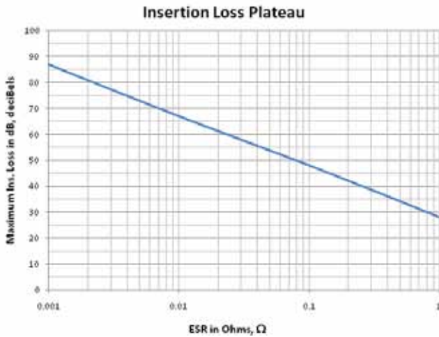
Figure 10. Maximum insertion loss versus ESR.
