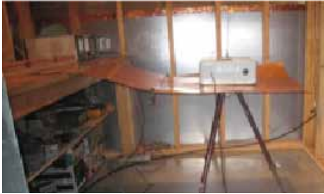
Figure 3a. MIL-STD-462 Notice 2 through MIL-STD-461E, RTCA/DO-160 through -160E, CISPR 25-2002 rod antenna set-up.
