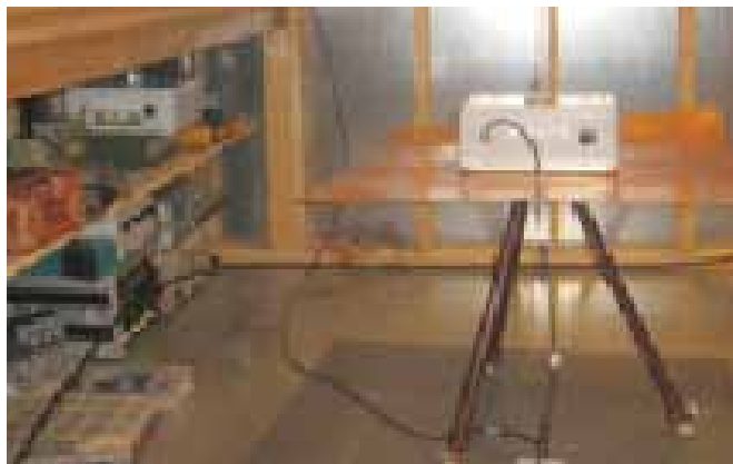
Figure 3b. MIL-STD-461F rod antenna set-up.
