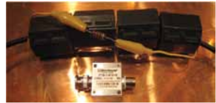
Figure 6a. Rf sleeves and resistor that place 270 Ohms between counterpoise and floor above 20 MHz, and isolation transformer that floats counterpoise.
