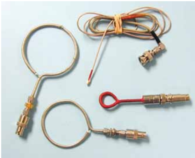
Figure 4. Examples of homemade H-field probes.
